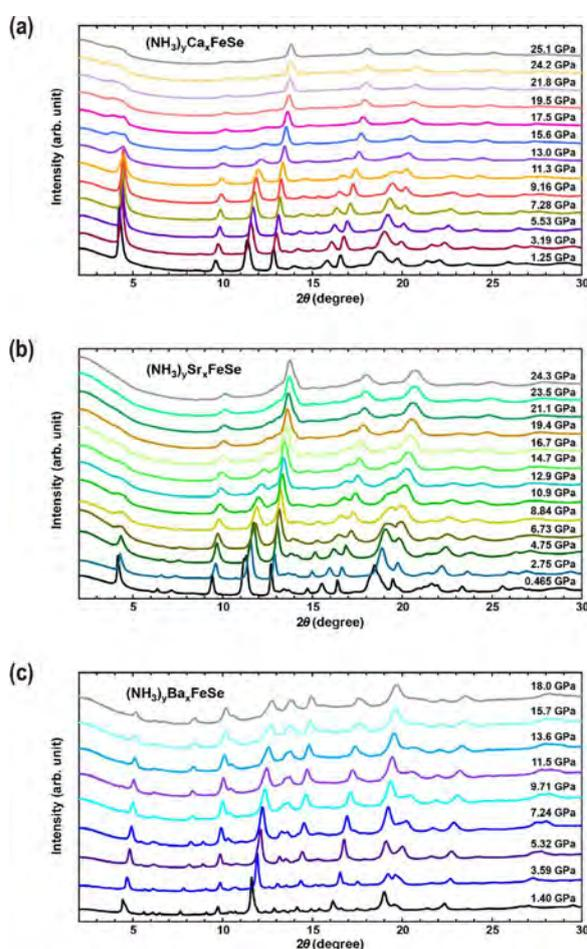
Fig. 2. Pressure-dependent XRD patterns for (a)  $(\text{NH}_3)_y\text{Ca}_x\text{FeSe}$ , (b)  $(\text{NH}_3)_y\text{Sr}_x\text{FeSe}$ , and (c)  $(\text{NH}_3)_y\text{Ba}_x\text{FeSe}$  [26].
