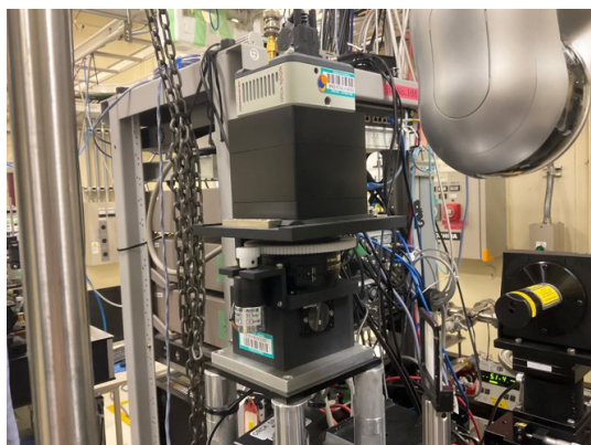
Fig. 4. Photograph of the permanently installed beam monitor for transmission imaging.
