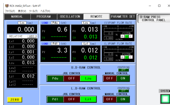
Fig. 2. Newly developed hydraulic control system with external command control function (REMOTE tab) at optical hutch.
