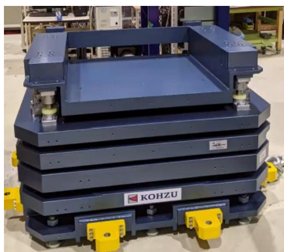
Fig. 2. Photograph of the portable 5-axis stage with a load capacity of 2,000 kg.
