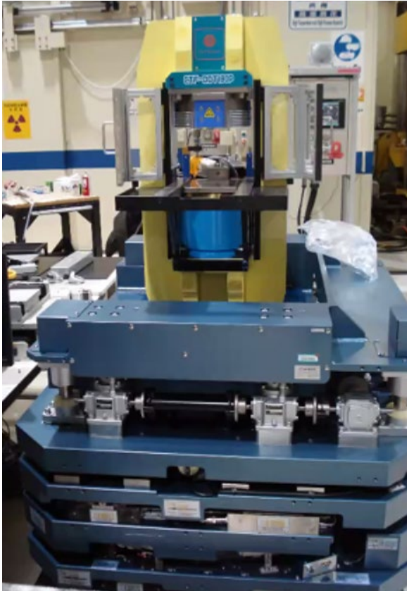
Fig. 3. Photograph of the large-volume press mounted on the 5-axis stage.
