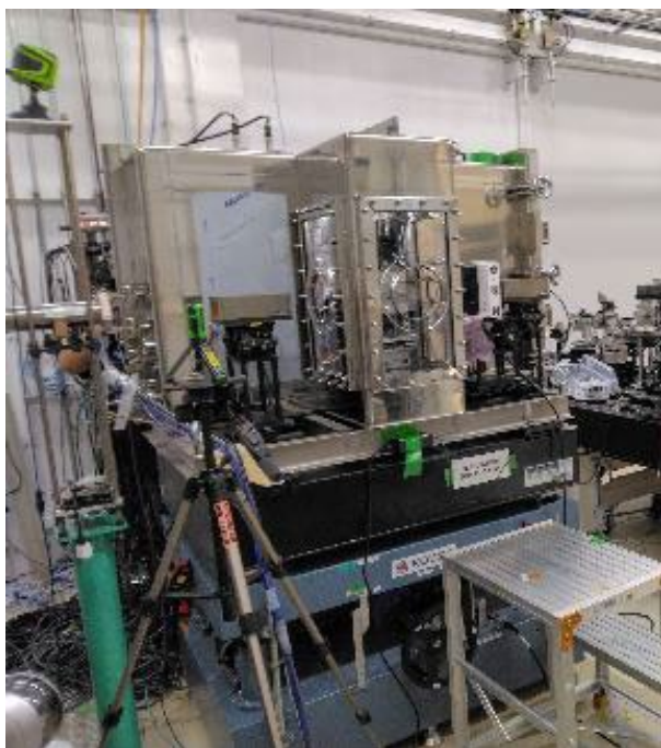
Fig. 1. Gas levitation system in the glove box at the BL22XU experimental hutch.
