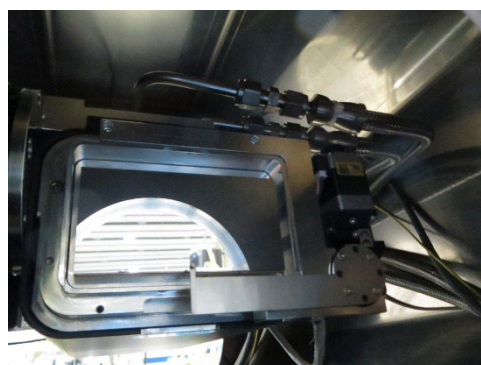
Fig. 4. Beamstop rotation drive mechanism in front of the WAXS detector.
