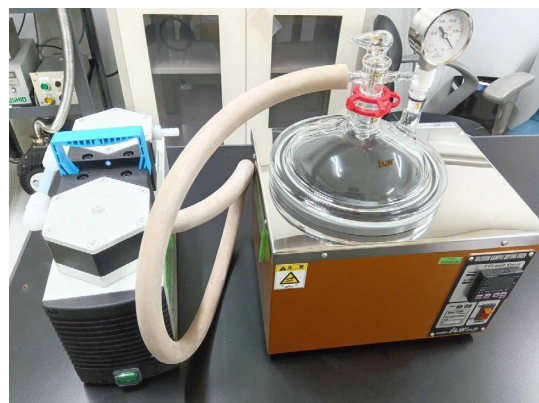
Fig. 4. Heating vacuum drying system.
