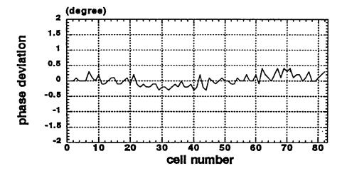
Figure 1. Phase deviation measured by Nodal shift method
