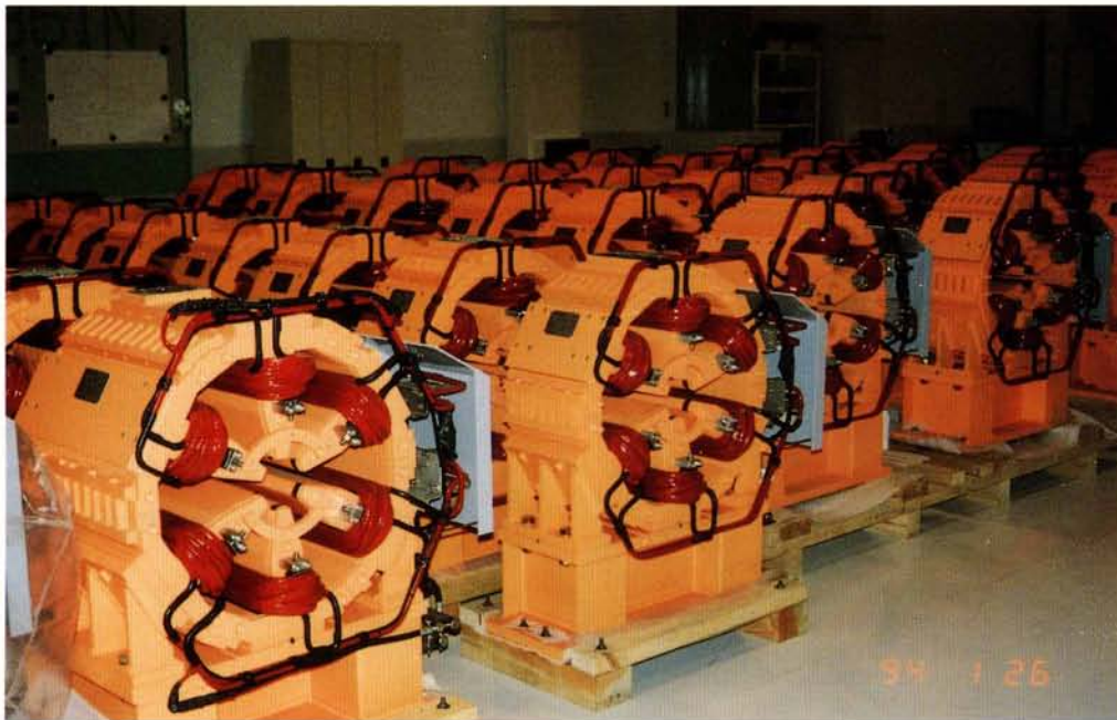
A number of quadrupole magnets for the storage ring were fabricated and waiting for the field measurement in the experimental hall.
