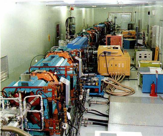
One unit cell of the storage ring magnet and vacuum systems was assembled to check and test mechanical and vacuum performance.
