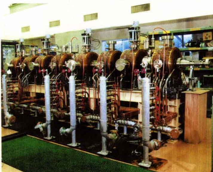
One unit of the RF cavities was assembled to check mechanical performance.
