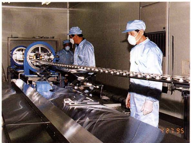
A unit of NEG pump was installed in the vacuum chamber of the storage ring.
