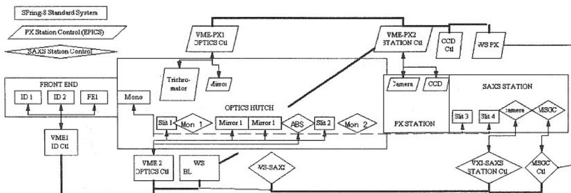
Fig. 4 Control Diagram of RIKEN beamline I
