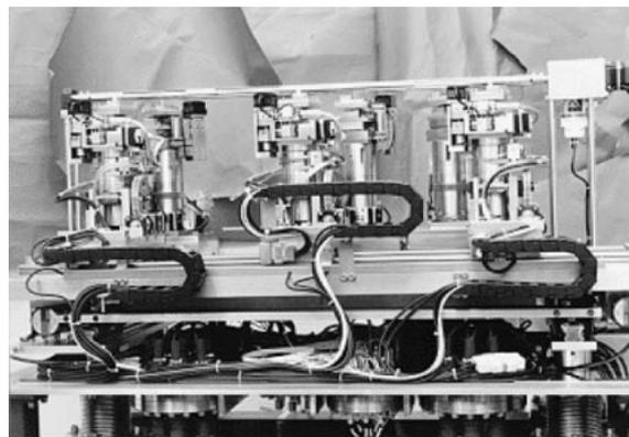
Fig.3 Side view of trichromator
