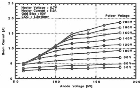
fig.4 Emission current characteristics versus anode voltage
