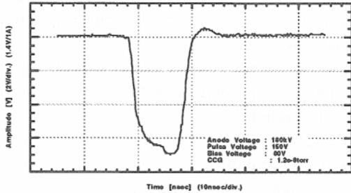
fig.2 The emission current at 10nsec pulse width
