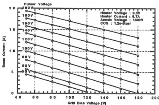
fig.5 Emission current characteristics versus grid voltage
