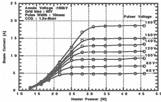
fig.3 Emission current characteristics versus heater power
