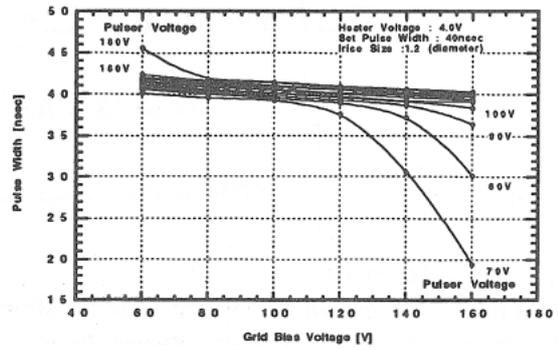
fig.6 Pulse width characteristics versus grid voltage
