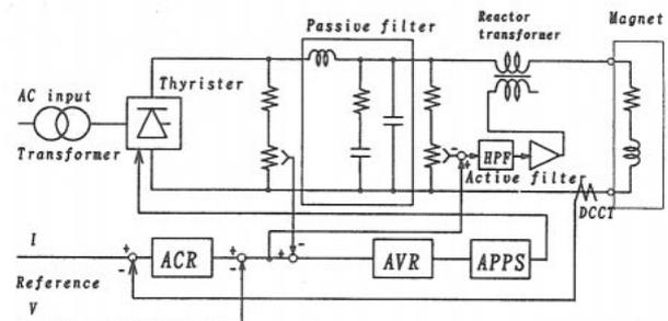
Fig.2 Block diagram of PS-BM. ACR and AVR : Automatic Current and Voltage Regulator, APPS : Automatic Pulse Phase Shifter, HPF : High Pass Filter.
