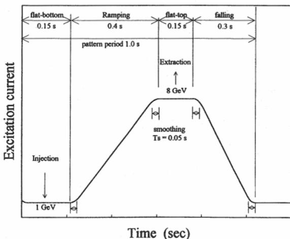
Fig.1 Excitation current pattern of lattice magnets
