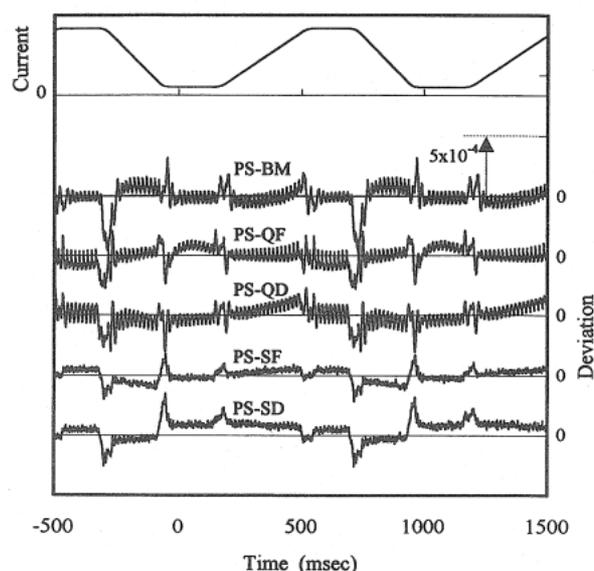
Fig.3 Current pattern and deviation of all power supplies; uppermost figure shows the output current pattern. Lower 5 figures show the deviation between the reference pattern and the output current for PS-BM, -QF, -QD, -SF, -SD.
