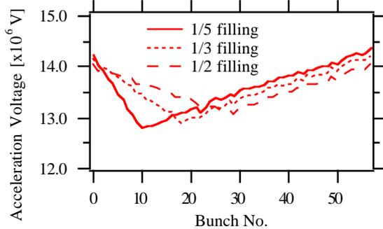
Figure 1. Amplitude of acceleration voltage vs. bunch number. The number of bunch per turn used in the simulation is 59 and first 1/5, 1/3 and 1/2 bunches filled with electrons. At equal filling, acceleration voltage is 13.5 MV
