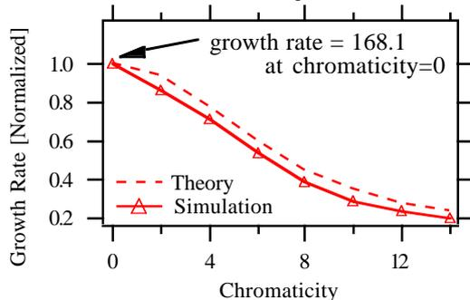
Figure 6. Growth rate of transverse multi-bunch instabilities driven by the model impedance with finite chromaticity.
