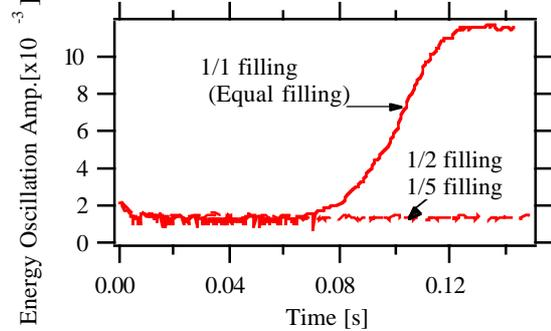
Figure 4. Simulation result for relative energy oscillation amplitude of a bunch for several filling patterns.
