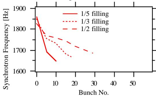
Figure 2. Synchrotron Frequency vs. Bunch Number from simulation result. Only bunches which have electrons are shown.
