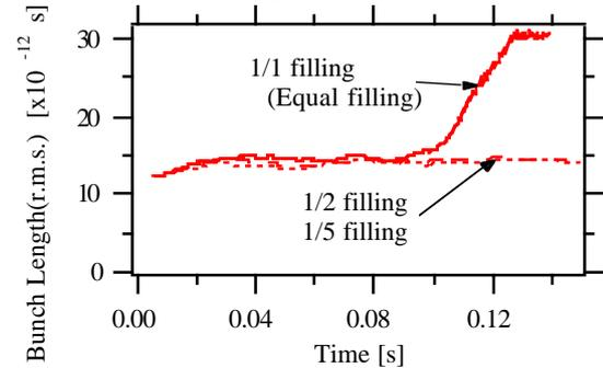
Figure 5. Simulation result for a bunch length for several filling patterns. The growth rate of the instabilities saturated by increase of the bunch length.
