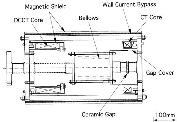
Fig. 2. Side View of the Current Monitor Assembly.
