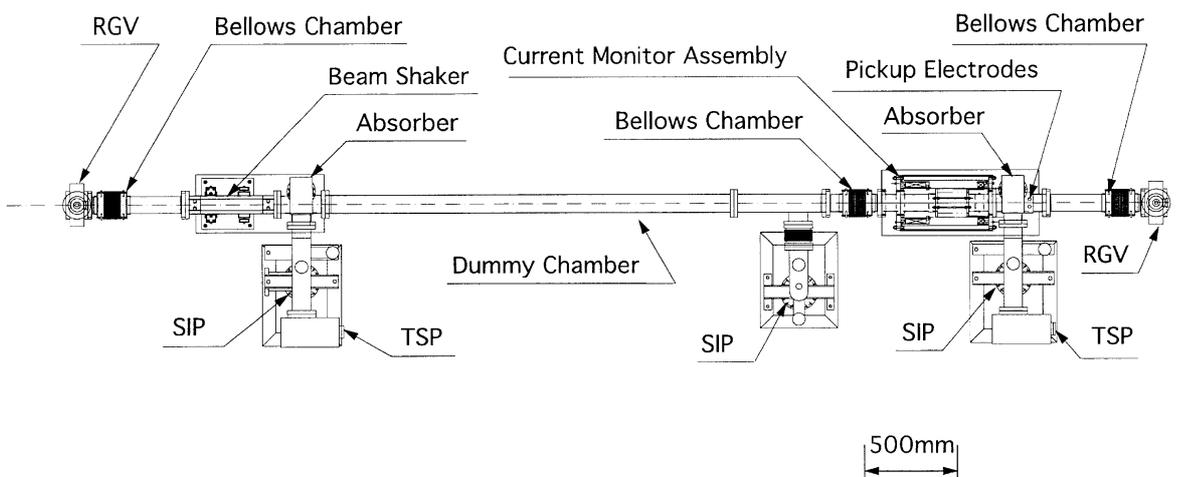
Fig. 1. The layout of the Beam Diagnostics Straight Section.
