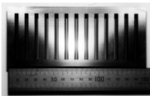
Fig. 7. Water distributor made of Si single crystal
