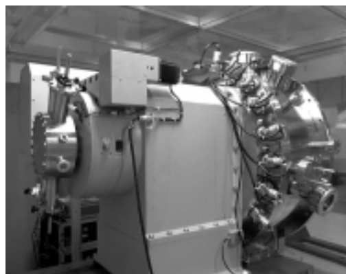
Fig. 3. Standard x-ray monochromator for undulator beamline
