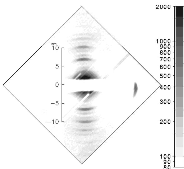
Fig.4: 2-dimensional image of SAXS experiment with a collagentarget at 9 keV X-ray beam.
