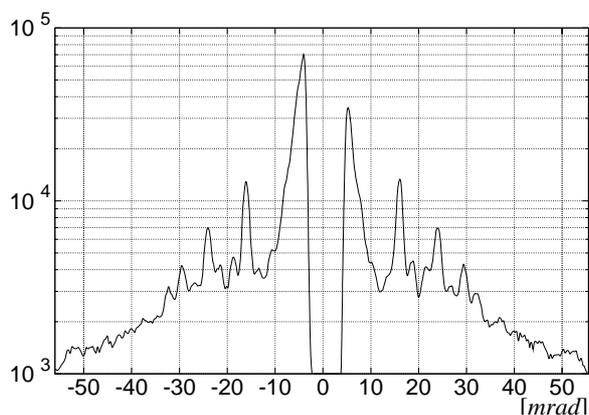
Fig.5: Angular distribution of SAXS experiment with a collagen target at 8 keV X-ray beam.
