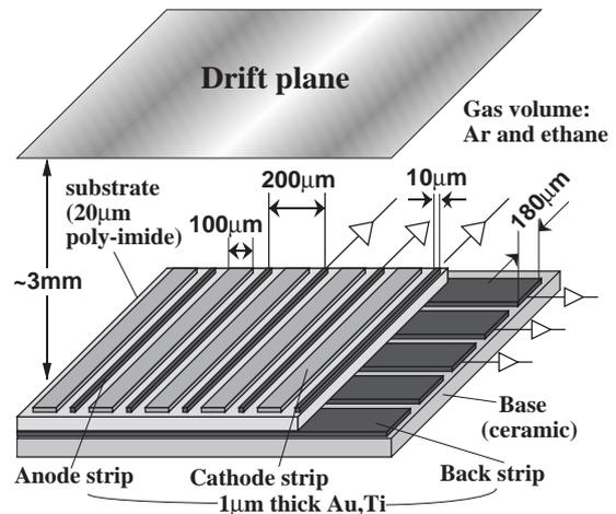
Fig.3: Schematic of the prototype detector with a  $50 \text{ mm} \times 50 \text{ mm}$  detection area.
