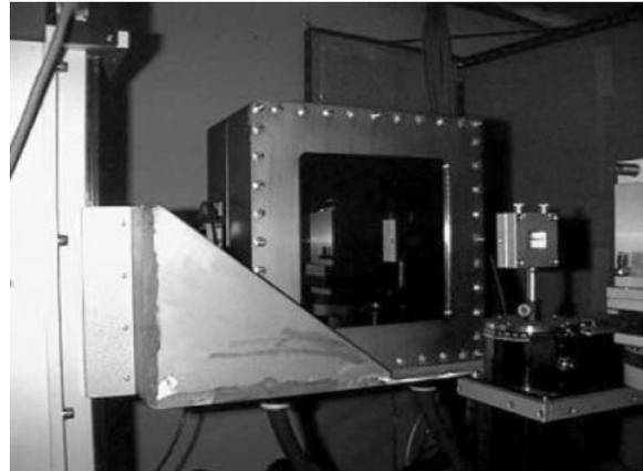
Fig.1: The Multiple Charge-Coupled-Device X-ray Detector constructed at EEV, UK.
