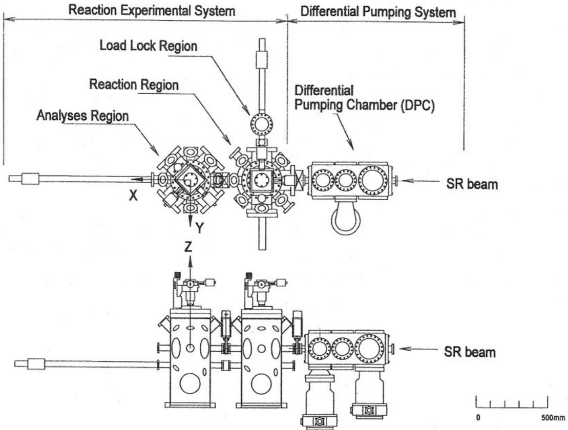
Fig 2. Schematic diagram of experimental station.
