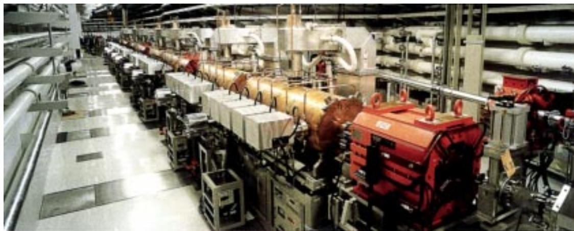
The RF cavities lined up at the synchrotron accelerate the electrons transported from the linac through a vacuum duct (right bottom) up to 8 GeV.
