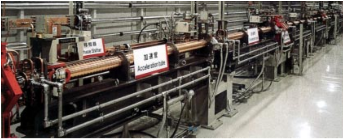
The linac accelerator column and its associated quadrupole magnets (red-painted) for beam-focusing. Before transported to the synchrotron, electrons are accelerated up to 1 GeV with this system.
