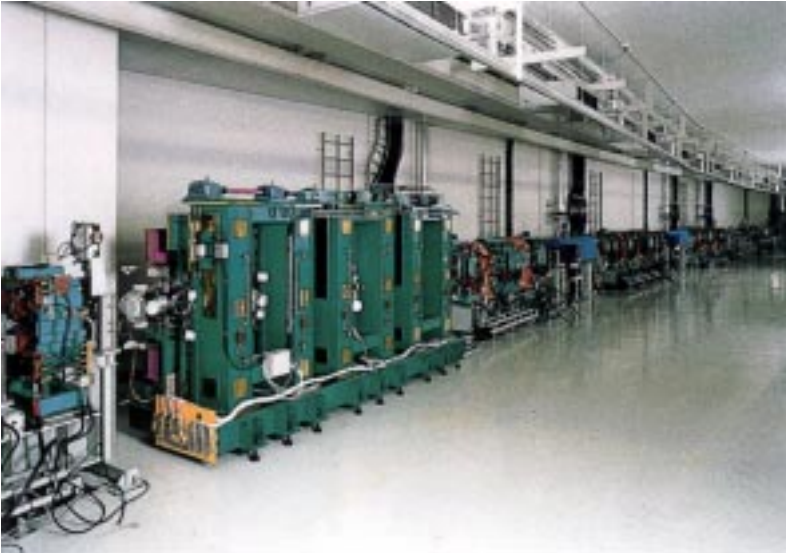
An in-vacuum undulator installed in the storage ring, in which the 8 GeV electron beam generates a highly brilliant x-ray beam of synchrotron radiation.
