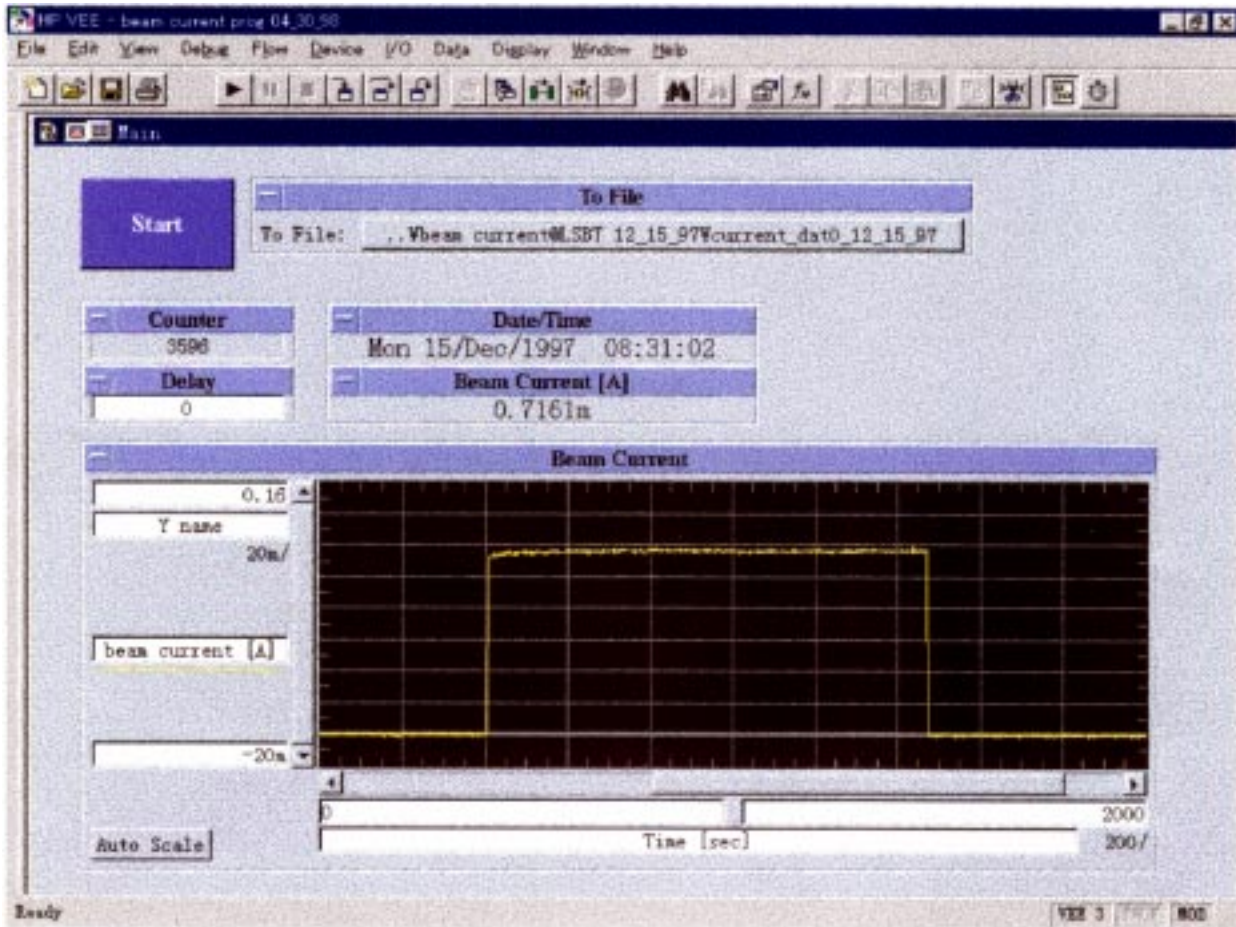
Fig.1, Linac output current injected into the synchrotron.
