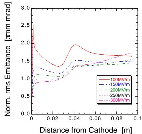
Fig. 1 The normalized rms emittance as a function of the distance from the cathode. Electric field gradient on the cathode is varied from 100MV/m to 300 MV/m.
