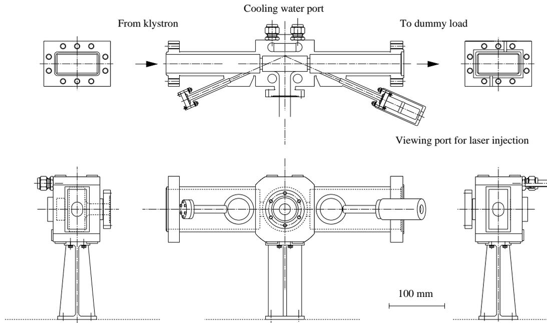
Fig. 3 The schematic of high power model cavity.
