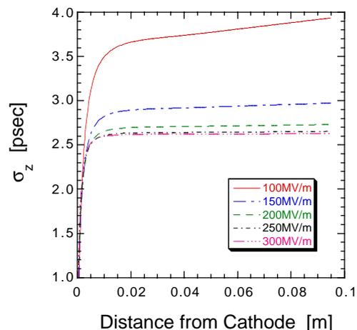
Fig. 2 The standard deviation of the bunch length as a function of the distance from the cathode.
