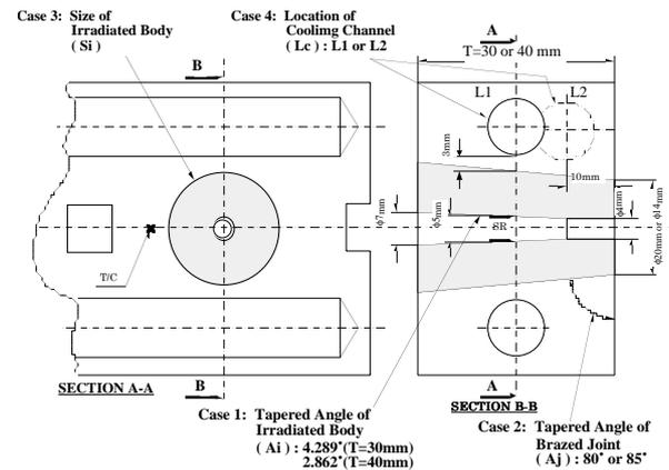
Fig.1. Parameters for the modification of fixed mask portion.
