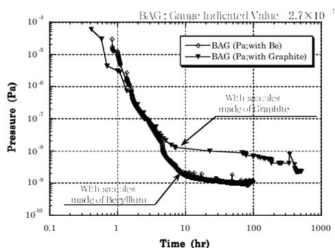
Fig.2. Pumping curves measured by BAG after 300 °C x 48 hours bakeout in both cases of with samples made of beryllium and with samples made of graphite.
