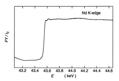
which limits the analytical resolution. In this study, we have attempted to measure EXAFS on the Nd K-edge (43.571 keV) in order to analyze the local structure in more detail.
