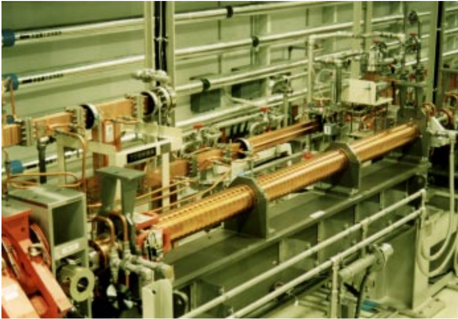
A part of injector linac, which accelerates an electron beam to 1 GeV.
