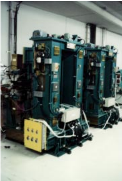
Twin-helical undulator for soft X-ray beamline BL25SU. Two helical undulator ( \lambda_u=120\text{mm} , N_u=12 \times 2 , E_{\text{photon}}=0.25\sim 4.5\text{keV} ) are placed in tandem for fast helicity switching.
