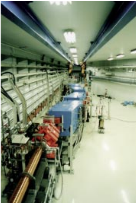
Beam energy analyzing system newly installed at the end of 1 GeV linac. The system consists of four rectangular bending magnets and beam monitors.
