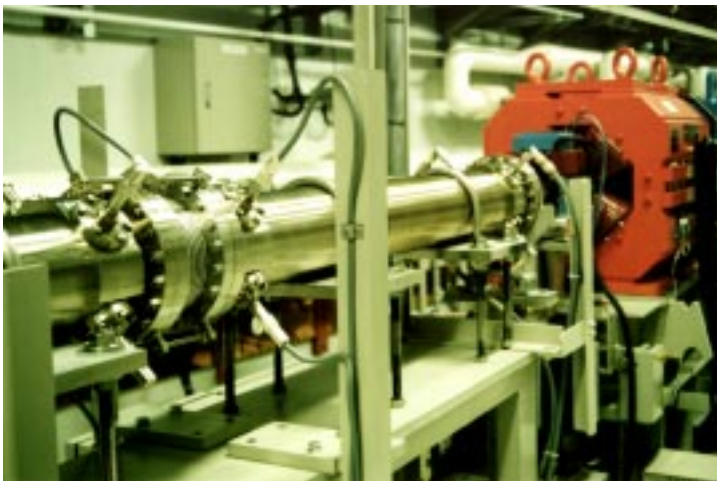
RF knock out electrodes installed in the synchrotron for single bunched beam operation. Four 1-m-long stripe-line type electrodes in a vacuum chamber generate electromagnetic force to remove electron beam from satellite RF buckets.
