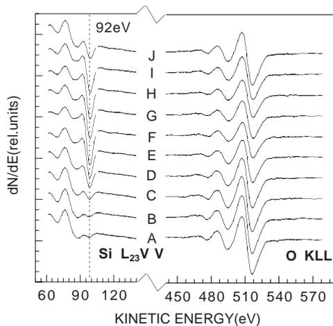
Fig. 2: Auger signal from irradiated with a dose of about 9,400 mA·min at 740°C. (A to C: non irradiated region, D to J: irradiated region)
