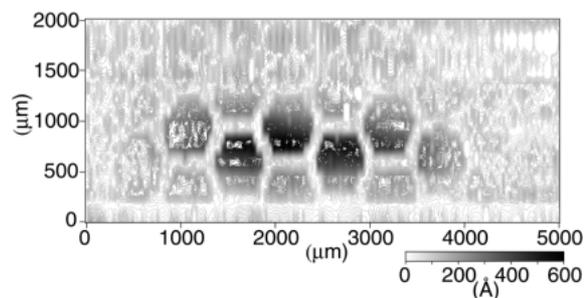
Fig. 1: Thickness profile of the SiO<sub>2</sub> film that was irradiated for a dose of about 9,400 mA·min at 825°C.
