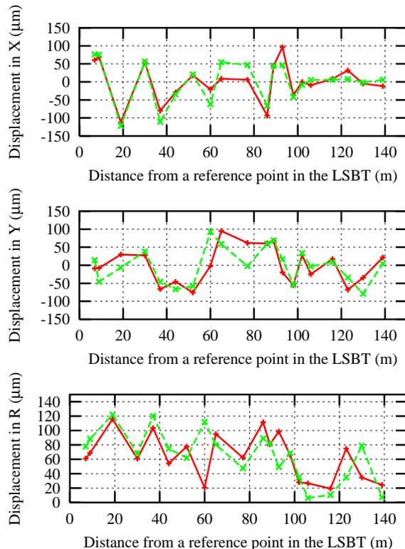
Fig. 1: Alignment error measured in 1995, just after installation of the magnets are finished. Measurements were performed along the on axis. These three data were measured in series. X is horizontal, Y is vertical, and R is radial direction.
