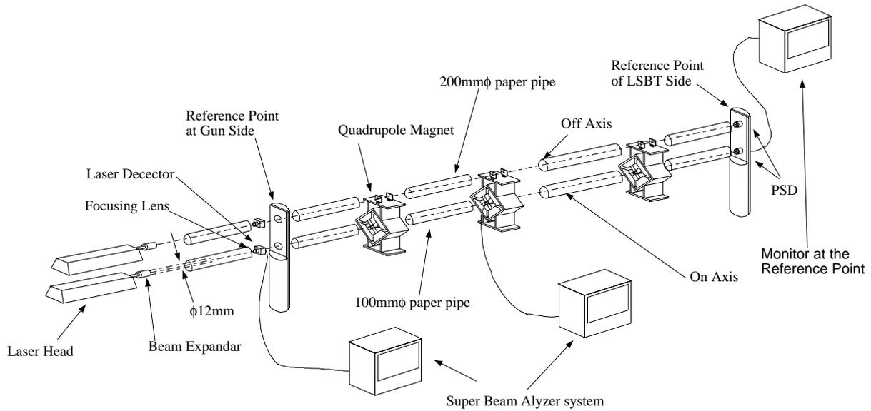
Fig. 3 The alignment error measurement system.
