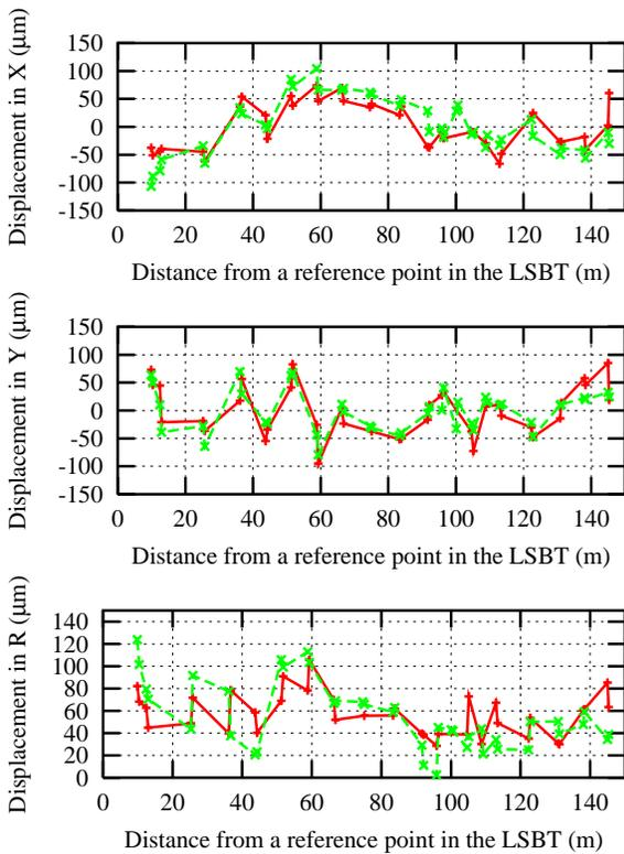
Fig. 2: Alignment error measured in 1998 summer. Measurements were performed along the shifted axis. Definition of X, Y and R is the same as Fig.1
