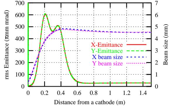
Fig. 7: Calculated emittances and beam sizes from cathode to Faraday cup. Parameters are the same as Table.1 except the initial rf phase of 60 degree.
