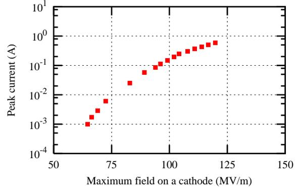
Fig. 2 Dark current from an RF cavity.
