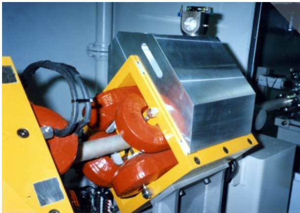
Fig. 5. Optic tool platform for quadrupole magnet alignment.
