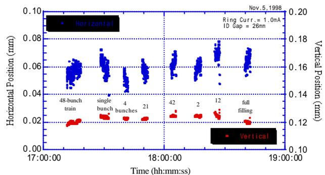
Fig. 2. Filling pattern dependence of XBPM@BL47XU.
