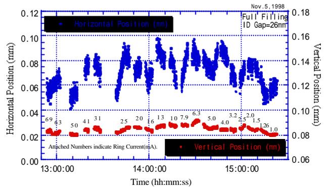
Fig. 1. Ring current dependence of XBPM@BL47XU.
