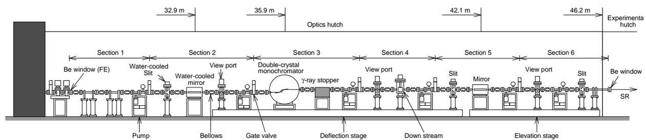
Fig. 1. Schematic view of BL01B1 transport channel.
