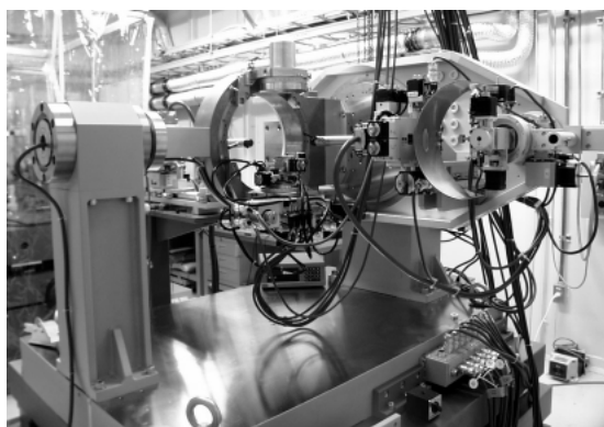
Fig. 3. Multi-axis goniometer for surface and interface structure analysis.
