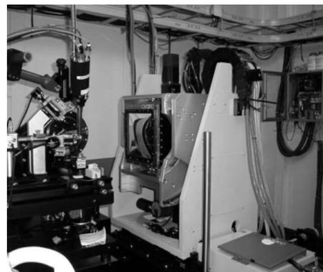
Fig. 3. CCD detector installed in the experimental hutch.
