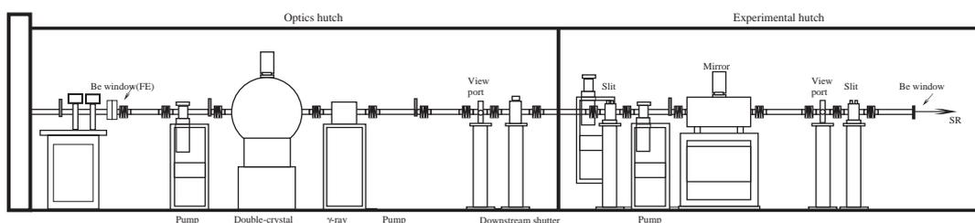
Fig.1. Schematic view of Optics Hutch of BL44XU.
