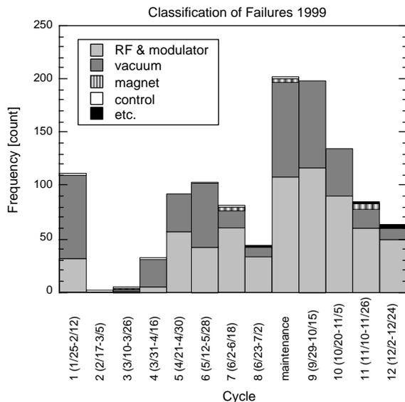
Fig. 1. Linac failure statistics for 1999.
