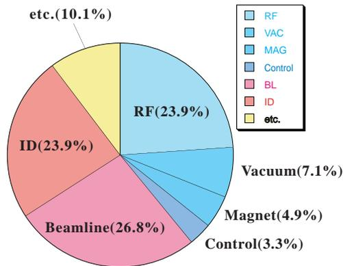
Fig. 2. The failure statistics of the storage ring in 1999.
