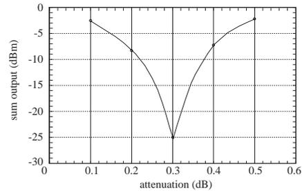
Fig. 3. The amplitude of the subtracted signal as a function of the attenuation of the strip line 4 signal.
