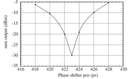
Fig. 2. The signal amplitude of the subtracted signal as a function of the position of the trombone.
