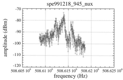
Fig. 5. The measured spectrum at the horizontal tune.
