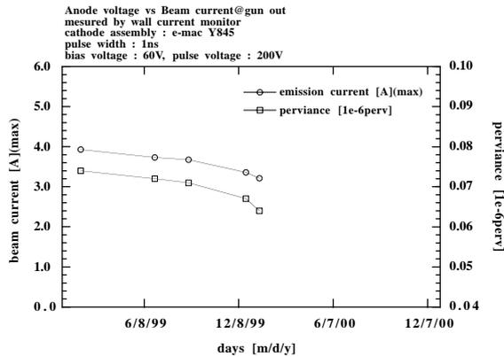
Fig.1. Curves of deterioration of beam current and perveance of electron gun.
