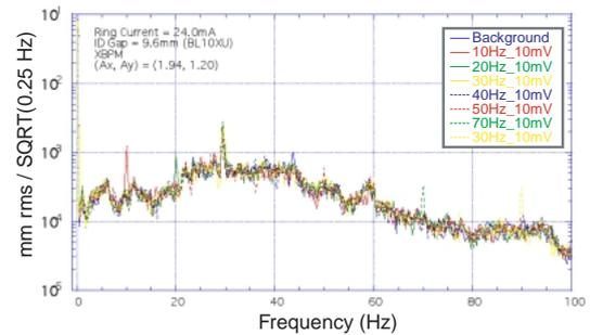
Fig. 4. FFT analysis of the vertical photon beam position. The frequencies of 10 and 20 Hz can be observed clearly, but the peaks are suppressed over a frequency of 40 Hz. The large peak seen at 30 Hz is due to real electron beam oscillation.
