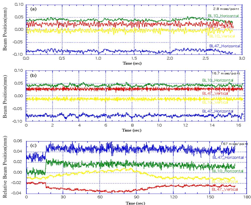
Fig. 1. Results of synchronous measurements using cellular telephones at BL47XU and BL10XU. The sampling rates are (a) 360, (b) 60 and (c) 6 samples/sec. In graphs (a) and (b), the steering magnets and ID were not changed. In graph (c), the electron orbit was steered with a steering magnet (the time is 16 sec.) and the ID gap of BL23 was changed from 40 to 80 mm (the time is 20 to 110 sec).
