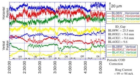
Fig. 3. Photon beam stability with and without periodic COD correction. Recently the correction scheme was improved, so there are no such steps as seen in this graphic.
