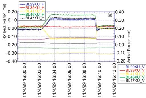
Fig. 2. Observation of the excitation of the dipole magnet in the experimental hutch of BL33LEP. The excitation current was applied with the maximum current from 16:03:40 to 16:09:20.
