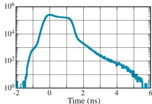
Fig. 2. Time response of the thick  $10 \times 10 \text{ mm}^2$  device to x-rays. The FWHM is about 1.6 ns.
