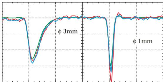
Fig. 3. Traces from  $\phi 1\text{mm}$  and  $\phi 3\text{mm}$  534X LC devices showing the response to 5.9 keV x-rays. The average over many events is shown (smooth curve) as well as two single-photon events to show an indication of the noise level. Scale: 100mV and 5ns /div.
