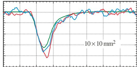
Fig. 1. Response of a  $10 \times 10 \text{ mm}^2 \times 185 \text{ um}$  APD to 5.9 keV x-rays. The average over many events is shown (smooth curve) as well as two single-photon events to show an indication of the noise level Scale: 50 mV and 5 ns /div.
