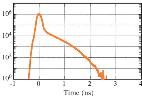
Fig. 4. Time response of the  $\phi 3\text{mm} \times 25 \mu\text{m}$  active thickness diode. Note the FWHM of 160 ps and the short tail.
