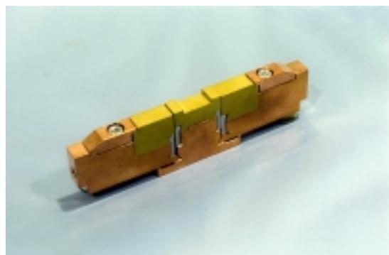
Fig. 4. Magnet unit for the in-vacuum helical undulator.
