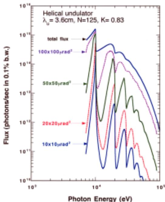
Fig. 2. Calculated spectral flux from the in-vacuum helical undulator for various slit apertures.
