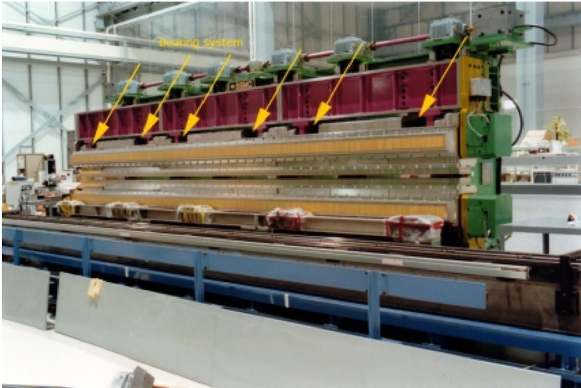
Fig. 5. Complete revolver just prior to installation into the SPring-8 ring.
