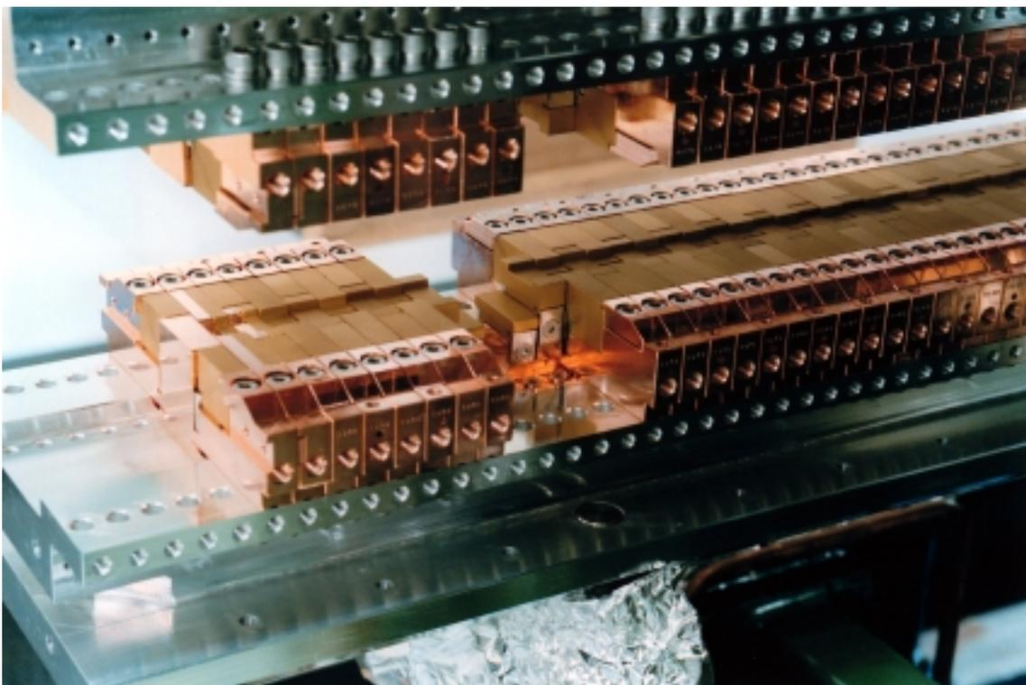
Fig. 3. Magnet arrays of the in-vacuum helical undulator under construction.
