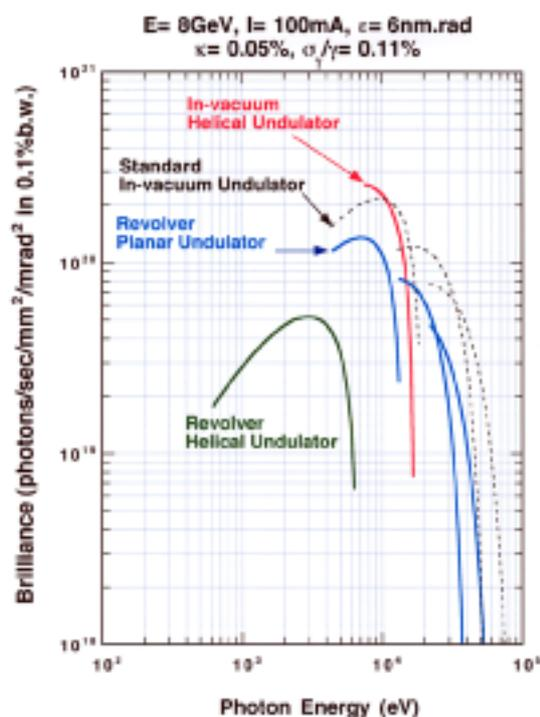
Fig. 1. Calculated spectral brilliances obtained from the in-vacuum helical undulator and the revolver (planar and helical undulators) in comparison with that of the standard in-vacuum X-ray undulator.
