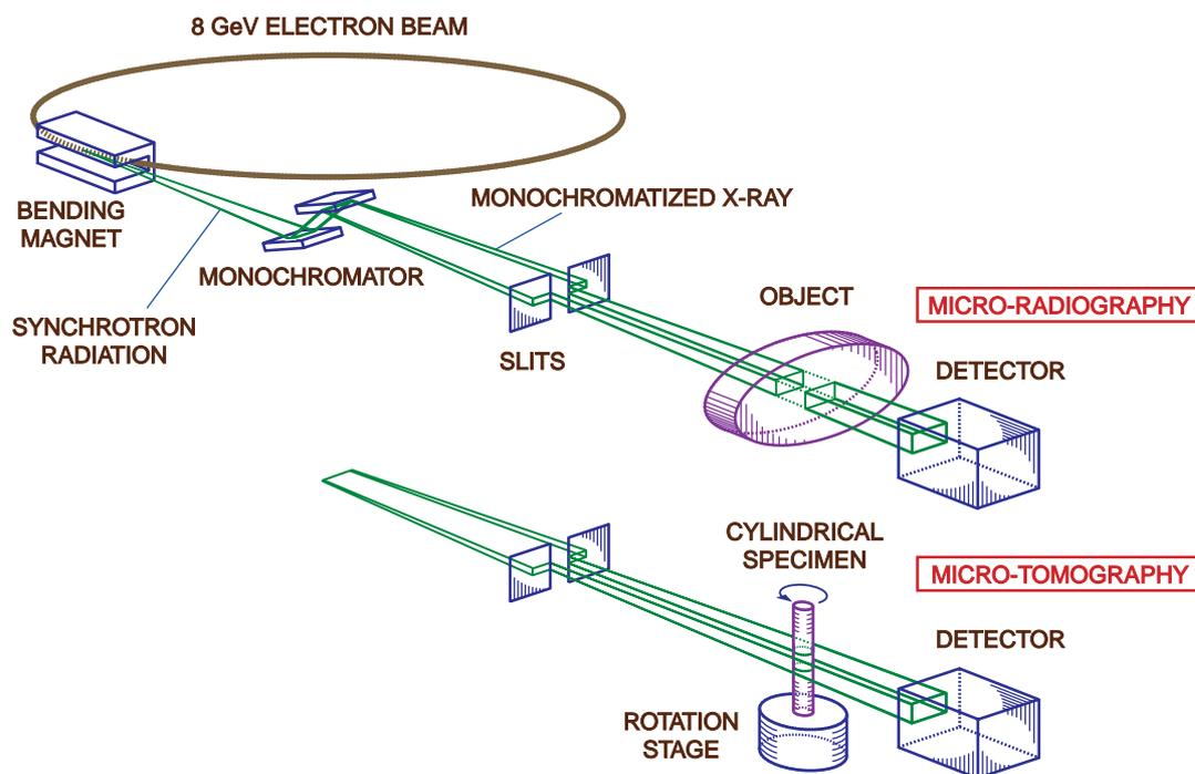
Fig. 2. Configurations of micro-radiography and micro-tomography.
