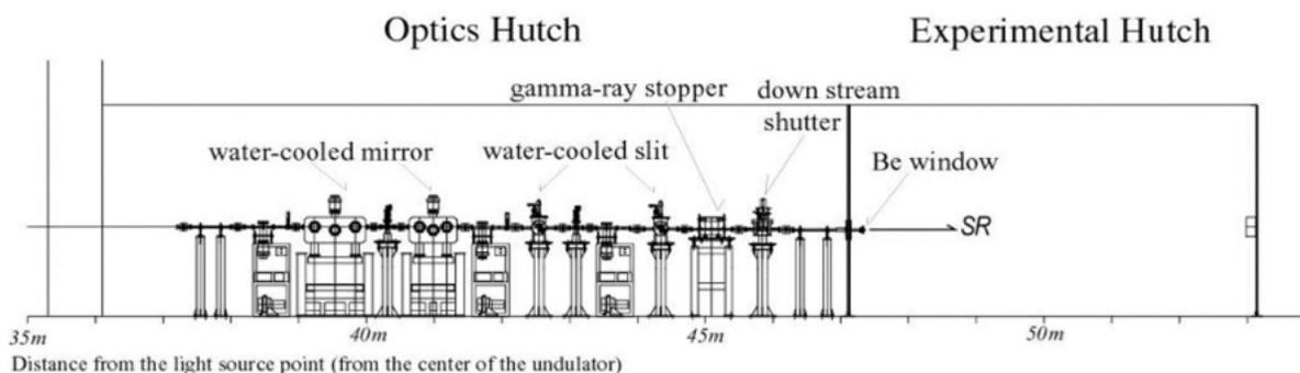
Fig. 1. The schematic view of the beamline.
