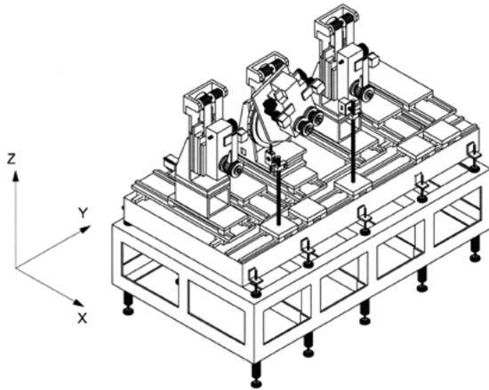
Fig. 2. Schematic view of the multi-axis precision diffractometer. Two  $\theta$ -goniometers and one 2axis- $\theta$  goniometer are mounted on the XY-carriers and a slit and a detector are set on the Y-carriers.
