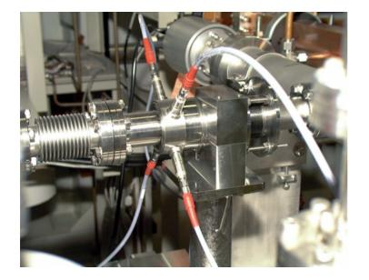
A prototype BPM for the SPring-8 linac was developed. Its output is high enough (14V/A) to obtain a micrometer resolution.
