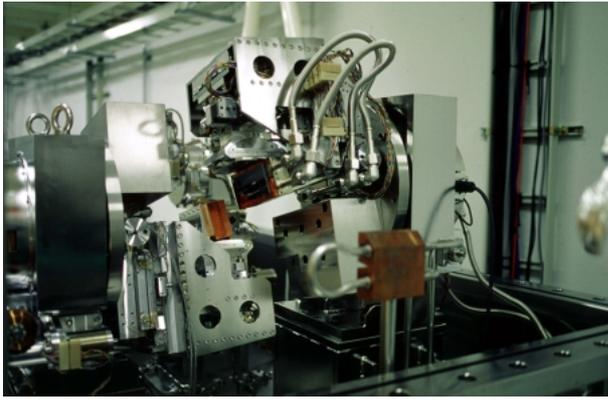
Si / YB<sub>66</sub> / Multilayer selectable monochromator was installed in BL15XU. The crystal or multilayer pair can be exchanged to cover a wide X-ray wavelength in conjunction with the revolver undulator.
