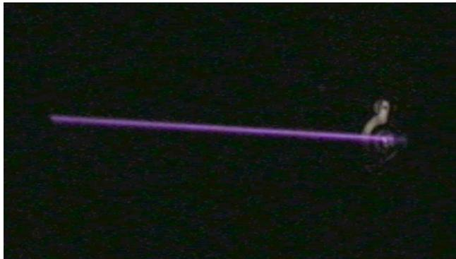
During the hutch radiation survey of BL40XU, a strong 8 keV X-ray traveled through the air in the experimental hutch. The fluorescence of air was seen clearly by eye.
