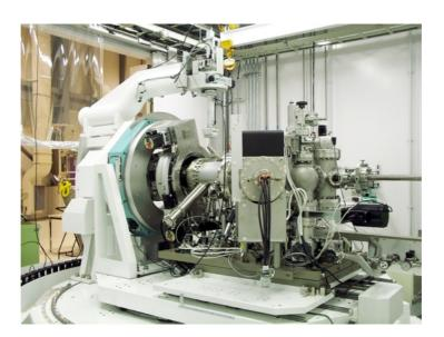
UHV surface X-ray diffractometer was installed at BL11XU. This diffractometer is designed for *in situ* studies on III-V group semiconductor surfaces.
