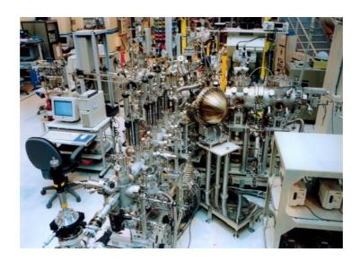
Surface reaction analysis apparatus at BL23SU composed of an electron energy analyzer, a supersonic molecular beam generator, a scanning tunnel microscope, quadrupole mass analyzers, a toxic gas supply system, etc. Photoemission spectroscopy and reactive molecular scattering experiments reveal surface reaction mechanisms induced by translational energy of incident reactant molecules on semiconductor-related materials.
