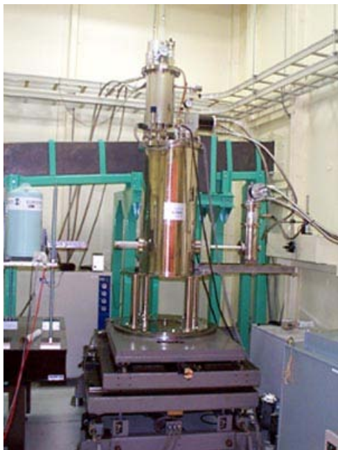
3-T superconducting magnet (switching time: within 5 seconds) with Refrigerator for sample (10 K ~ 300 K)
