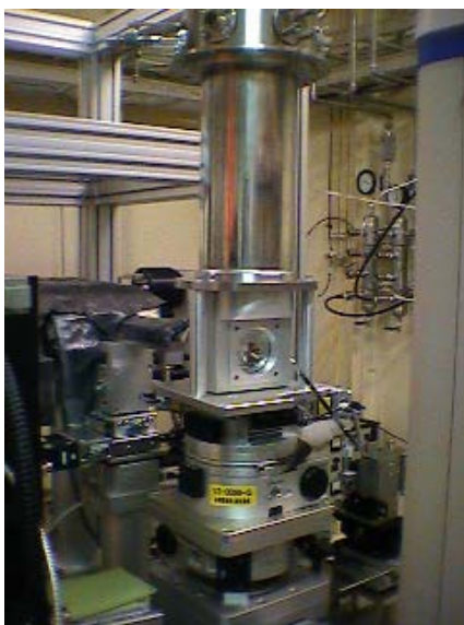
Fig.4. A cryostat with DAC mounted on the \omega stage goniometer
