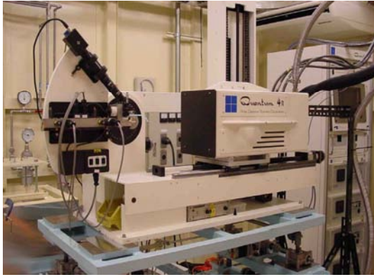
The ADSC Quantum 4R CCD detector for PX
