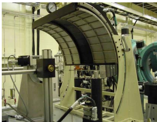
Curved image plate stage for PXD
