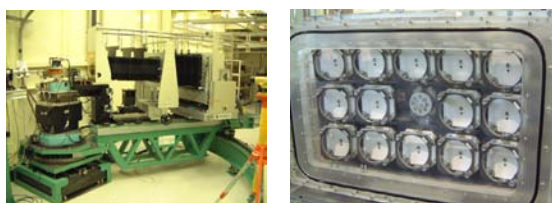
Fig.3. The 4-K cryostat and carrier (upper), and the 15-element multiple analyzer system (lower)
