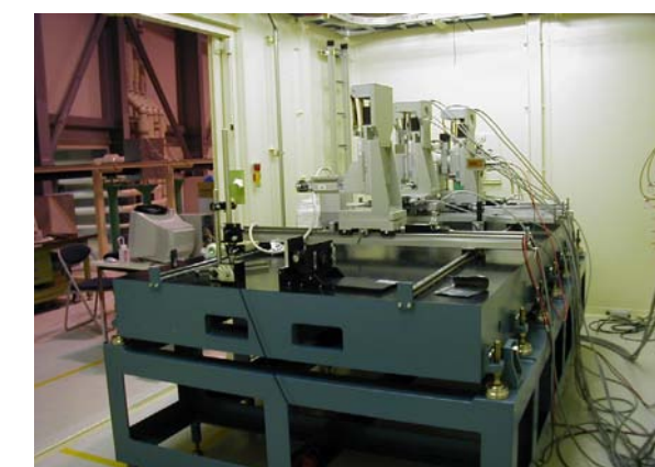
Versatile high-precision diffractometer for X-ray microscopy at the experimental hutch I
