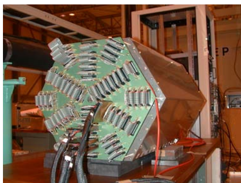
Time projection chamber tested beside BL33LEP
